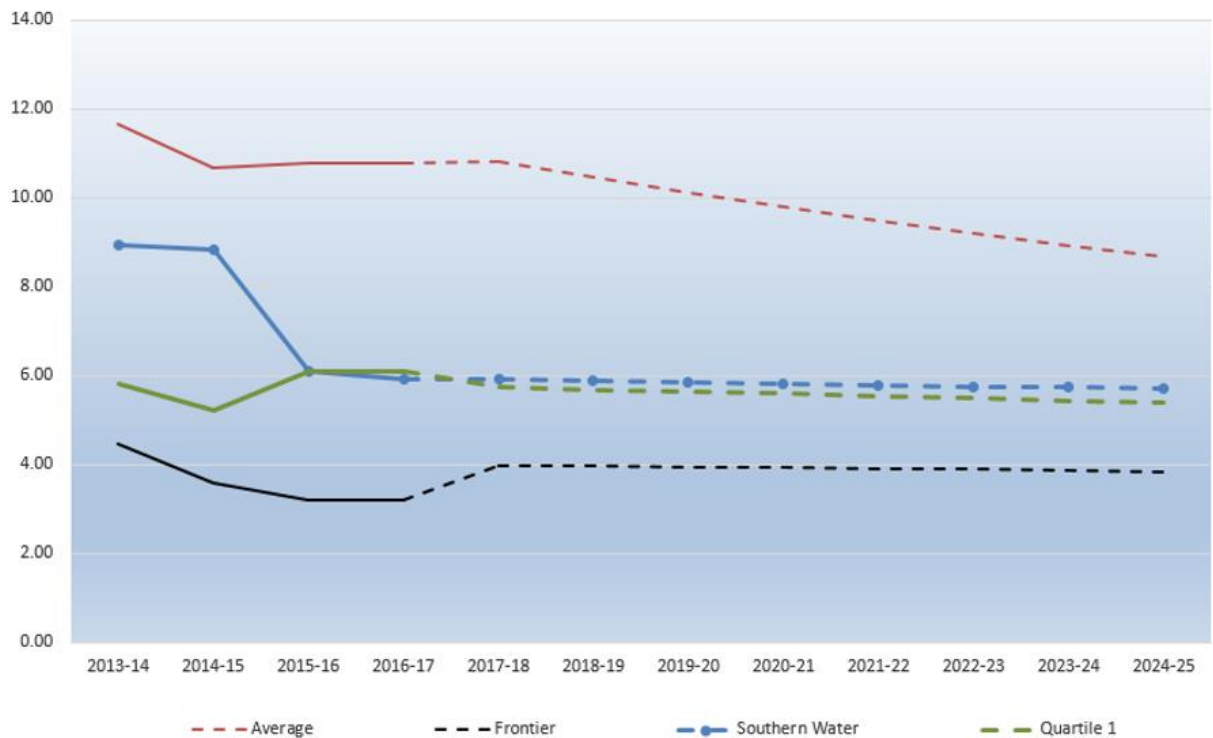
Figure 4: Sewer collapses (including rising main failures) 2013-2025
